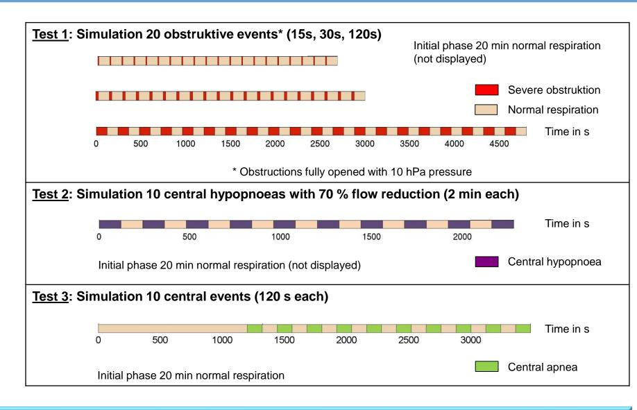
Draft test method for automatic pressure control of APAP devices.
